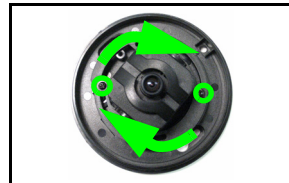
Figure 2.0 Loosen the screws and rotate the ring
