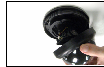
Figure 4.0 Attach the dome cover and screw the dome ring onto the base
