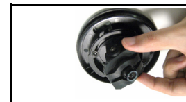
Figure 3.0 Loosen the screws and adjust the angle of the lens
