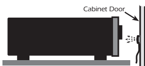
Fig. 5b IRE-2.0 attached to inside of cabinet door directly opposite IR sensor window
