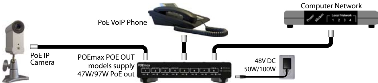
Figure 1 - POEmax switch as PoE power source: connect POEmax to power supply, computer network, and PoE powered devices such as wireless access points, VoIP phones, and IP cameras (NetMedia iViewHD).
