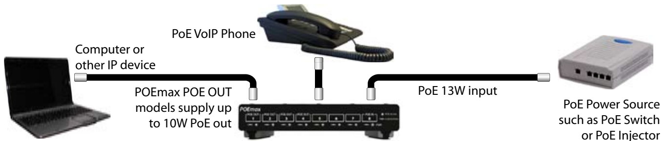
Figure 2 - POEmax as PoE-Powered switch: connect POEmax POE IN to a PoE switch/injector. POEmax will operate as a network switch. POE OUT models can rebroadcast power to other PoE-Powered devices such as VoIP phones and IP cameras.
