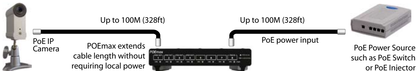
Figure 3 - POEmax as PoE-Powered data/cable extension: connect POEmax POE IN to PoE switch/injector. POEmax will extend Ethernet cable length up to another 100M. POE OUT models can still redistribute any available PoE power.
