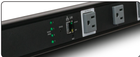
Front Panel with Status Indicators, Ethernet port, and Reset Button
