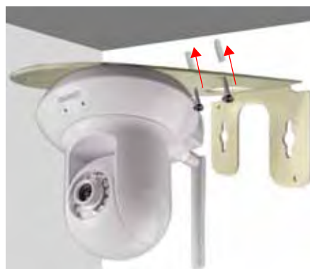
Figure 2.3 Secure camera and bracket to ceiling (LNZ4001 Series)
